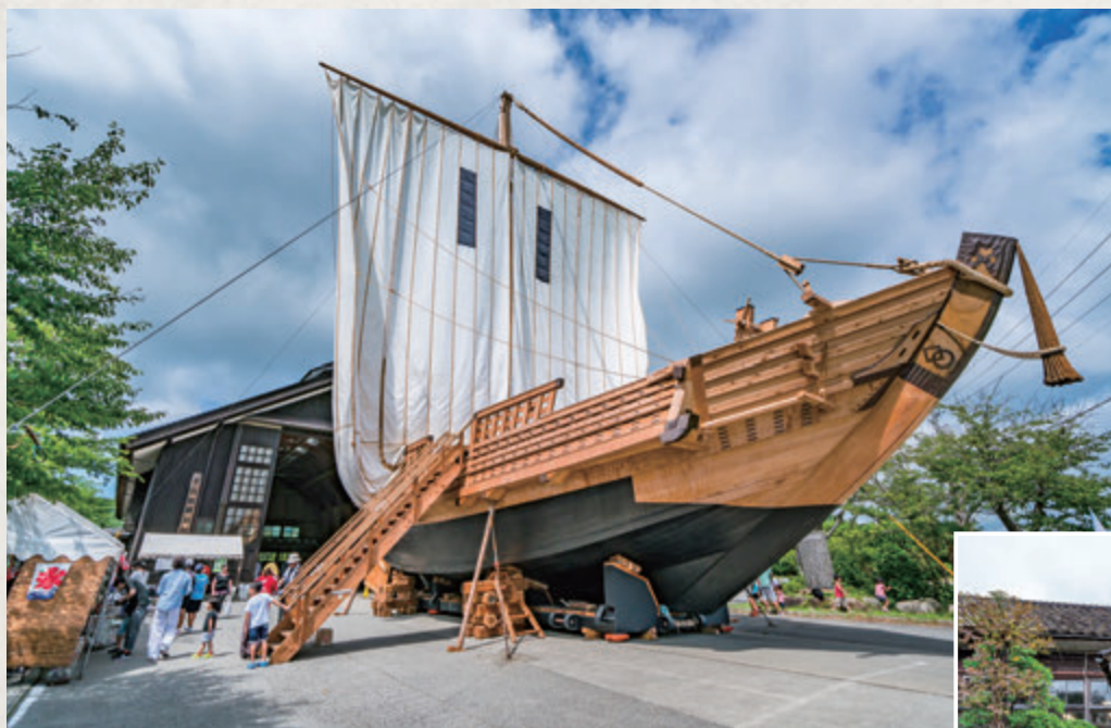
Sengokubune "Hakusanmaru" Sengokubune is a large wooden trading ship with a cargo-carrying capacity of 1000 koku (150 tons, "sengoku" in Japanese). Length: 23.75 m Stern height: 6.61 m Tonnage: 77 tons (512 koku)
